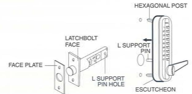
Insert the 2 hexagonal posts into the upper and lower holes of the front body and place the escutcheon on. Position the front body onto the door.
